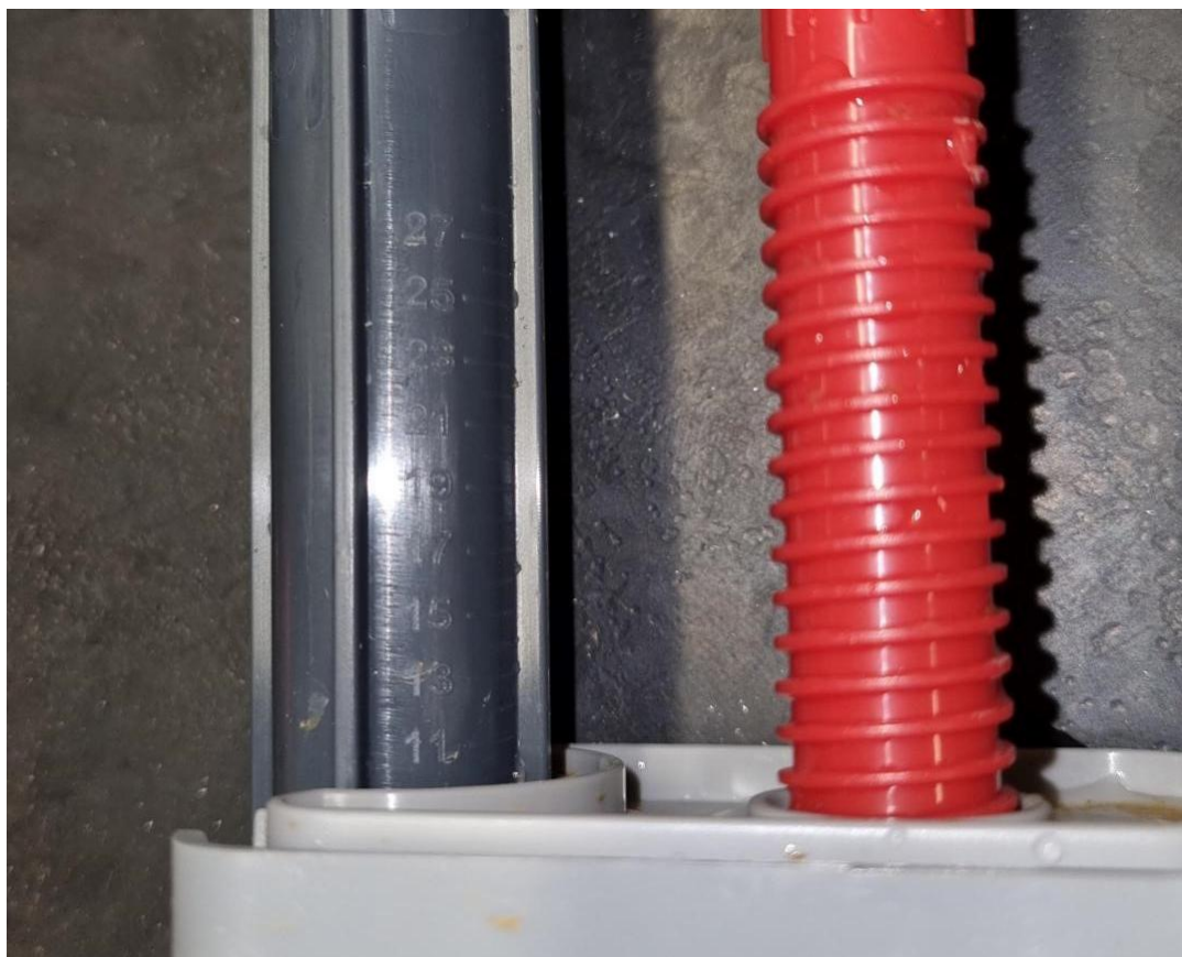
Float level between 9 and 11. The correct position for reading the level
